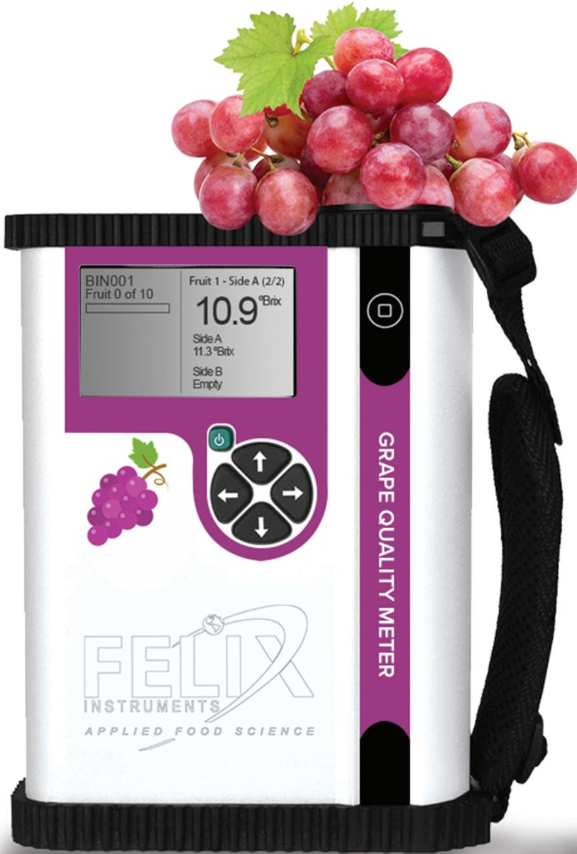
The F-751 Grape Quality Meter precisely and non-destructively measures **Brix, pH, and titratable acidity**, which are key indicators of table grape quality and ripeness. Utilizing near-infrared (NIR) technology, the F-751 enables users to accurately assess the readiness for harvest and evaluate grape quality on the spot.
